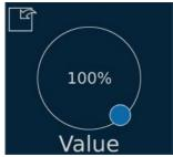
NOTE! The sent value to the device in the event of an event opposed to change of scene or program master is sent after selecting the set value with the slider and releasing it – the change is not smooth.
