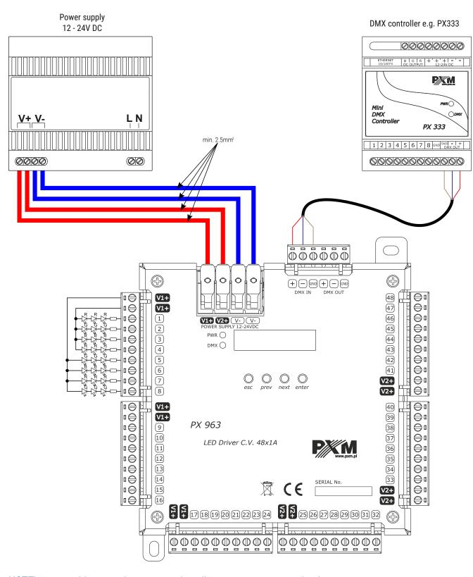
NOTE! Power cables must be connected to all input connectors on the device.
